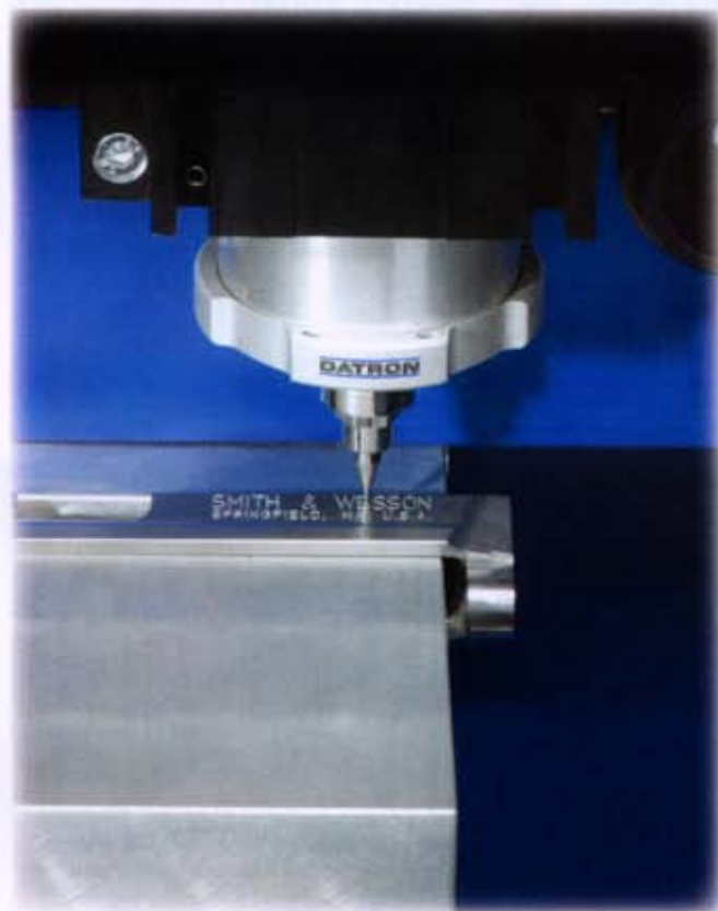
The Datron Dynamics mechanical engraver etches logos and other identifying marks into stainless steel
